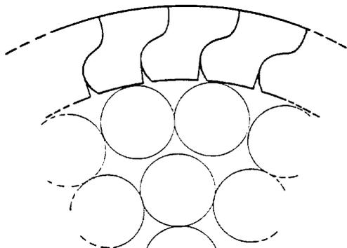
Figure 1. Sector of a cross-section of compact conductor
