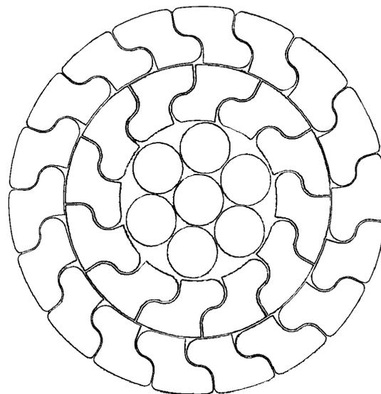
Figure 2. Cross-section of an AERO-Z<sup>®</sup> conductor
