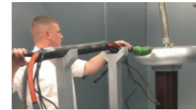
AC voltage testing up to 200 kV
